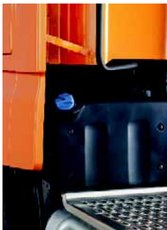
Adblue-Tank: immer in Motornähe
